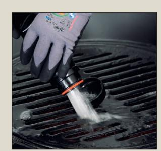
Empty and clean the recovery tank and float system.
