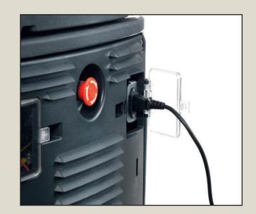
Disconnect battery charger and store the cable in the storage compartment located under the seat.
