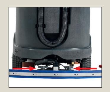
Install the squeegee and fix it by using the two knobs.
