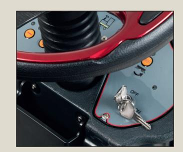
Insert the operator key and start the machine.
