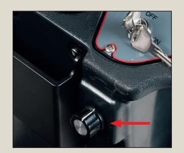
Adjust the maximum speed with the speed adjustment dial.
