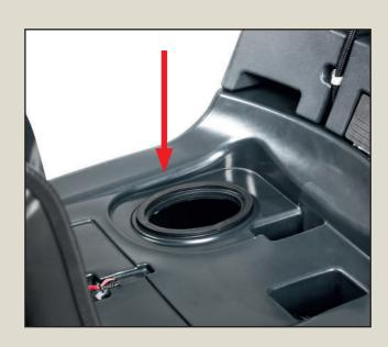
Fill the solution tank with fresh water and add low foam detergent according to needs.
