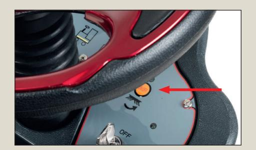
Switch brush motor button on.
