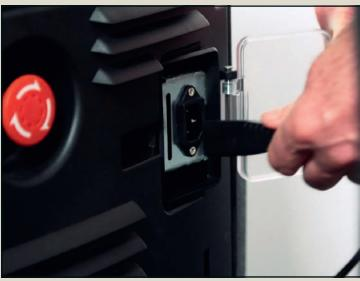
Connect the battery charger cable to the machine and the wall socket.
