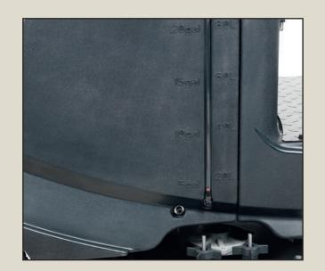
Solution level indicator is on the side of the tank showing current level.
